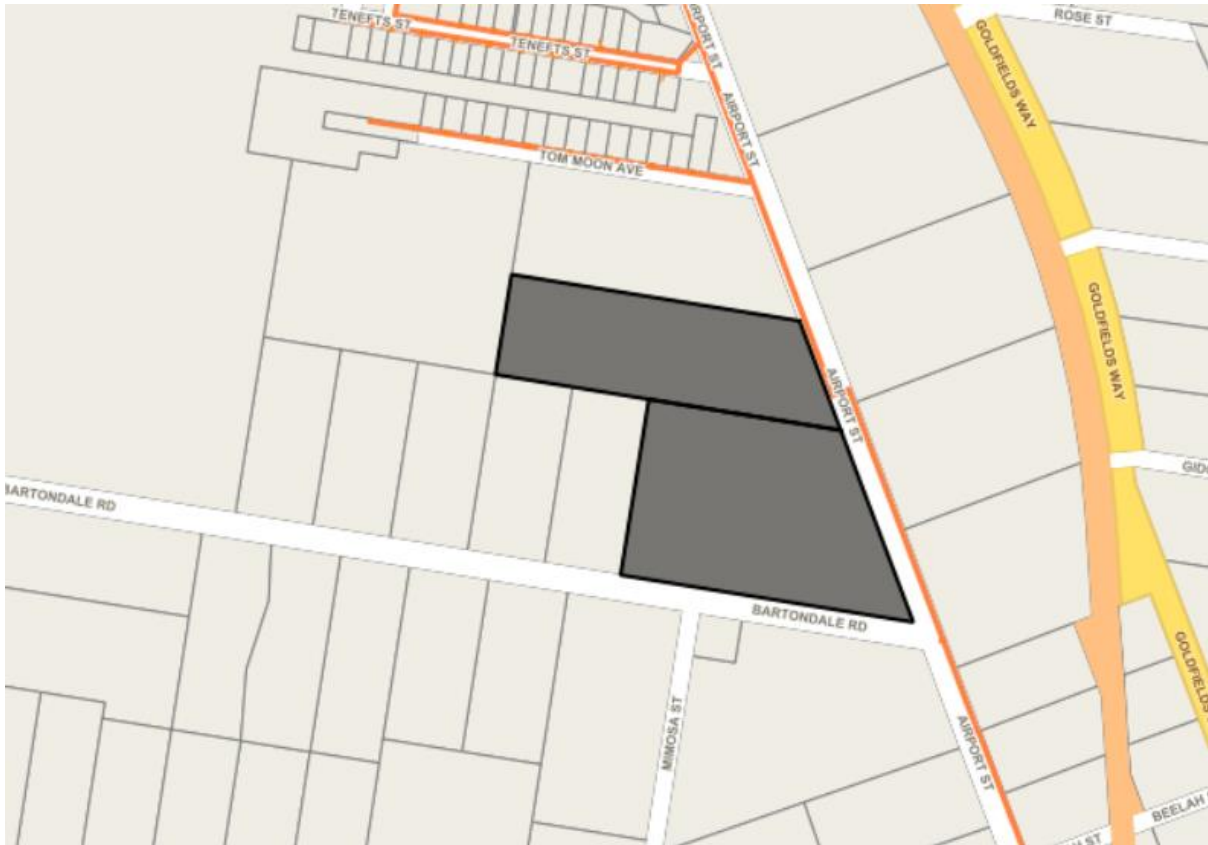
Figure 10: Gas services adjacent to the development site
