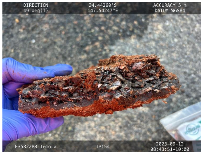
Photograph 7: Asphalt fragment in TP154
