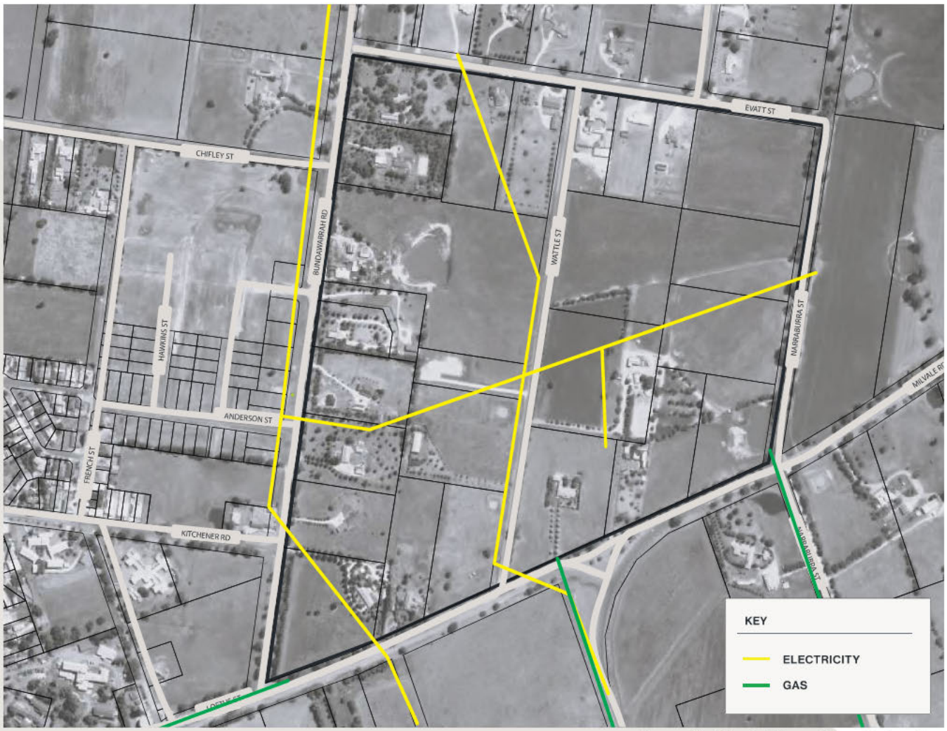
Figure 17 | Electricity and Gas Network
