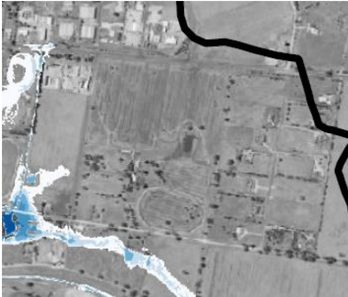
Figure 68: Land affected by the 1% AEP as identified by the Temora Flood Study 2019
