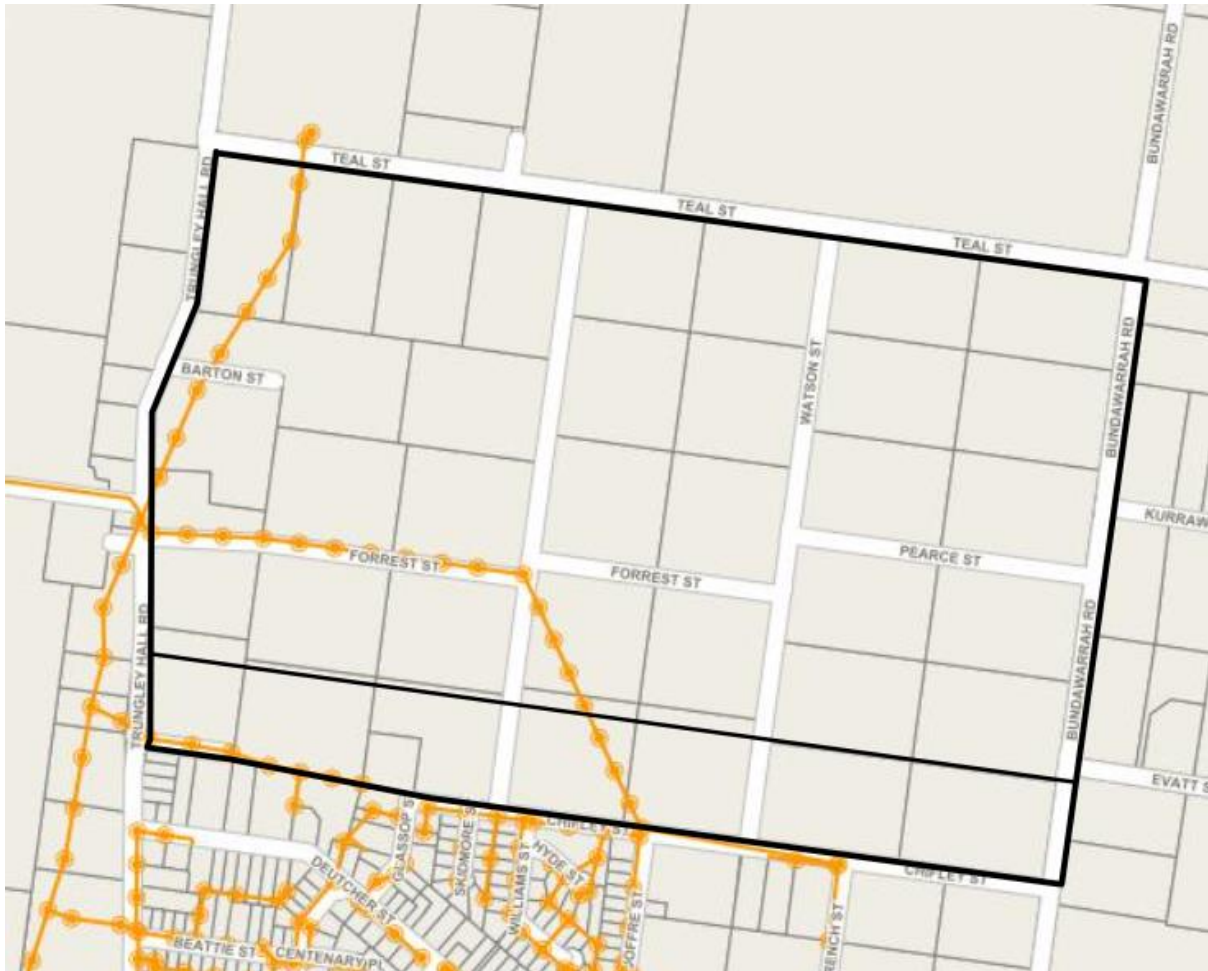
Figure 56: Northern fringe and Chifley Street sewer infrastructure
